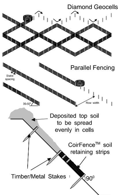
**Soil Stabilisation** *CoirFence™* is a new system designed for easy creation of retaining geocells, and stabilisation fencing, on embankments where top soil is vulnerable to slippage during vegetation establishment.
