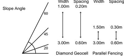
The above figures are given for guidance only. Factors such as fill type, shear strength of underlying ground and severity of erosion forces must be taken into consideration
