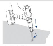
Position the TL-P1 onto matting, apply slight downward pressure and activate drill
