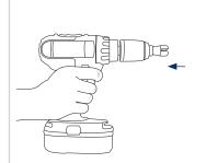
Insert the TL-P1 chuck into drill making sure it is secure
