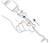
Place the circular head of the TL-P1 into the TL-P1 chuck and twist 90° into position
