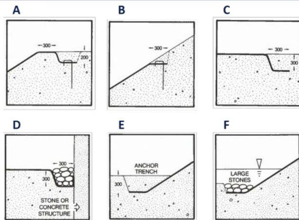
Fig 7: Alternative anchorage
